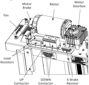
Figure 6-6 (wires not shown)
