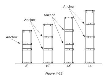
The 1st option is to use the optional tower brace that attaches to the sides for the tower. There are brackets that attach to a structure. Then the brackets are fastened together.
