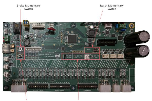
Service Momentary Switch 3X Permanent Cuttable Switches
