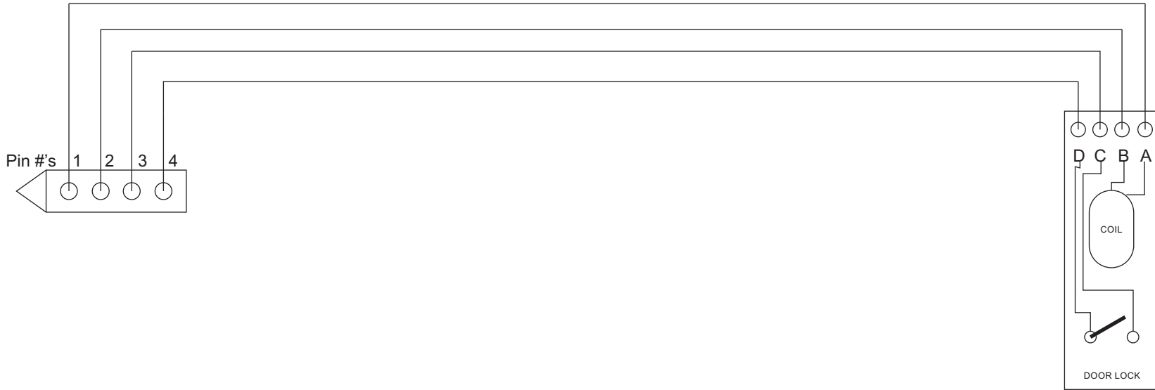
Typical Hall Call Station Diagram { } Indicate Pin Number
