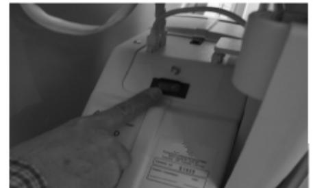
If the LED is not GREEN, turn the unit off and recheck all wire plugs and safety sensors. Turn on the RED ON/OFF Switch and recheck the LED cycle. When the LED remains GREEN, the lift is ready to operate.
